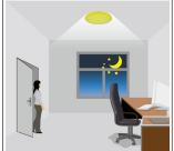
With ambient light less than daylight threshold, the lamp will be on 100% when someone enters the room
