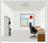
With ambient light more than daylight threshold, the lamp does not switch on when someone enters the room
